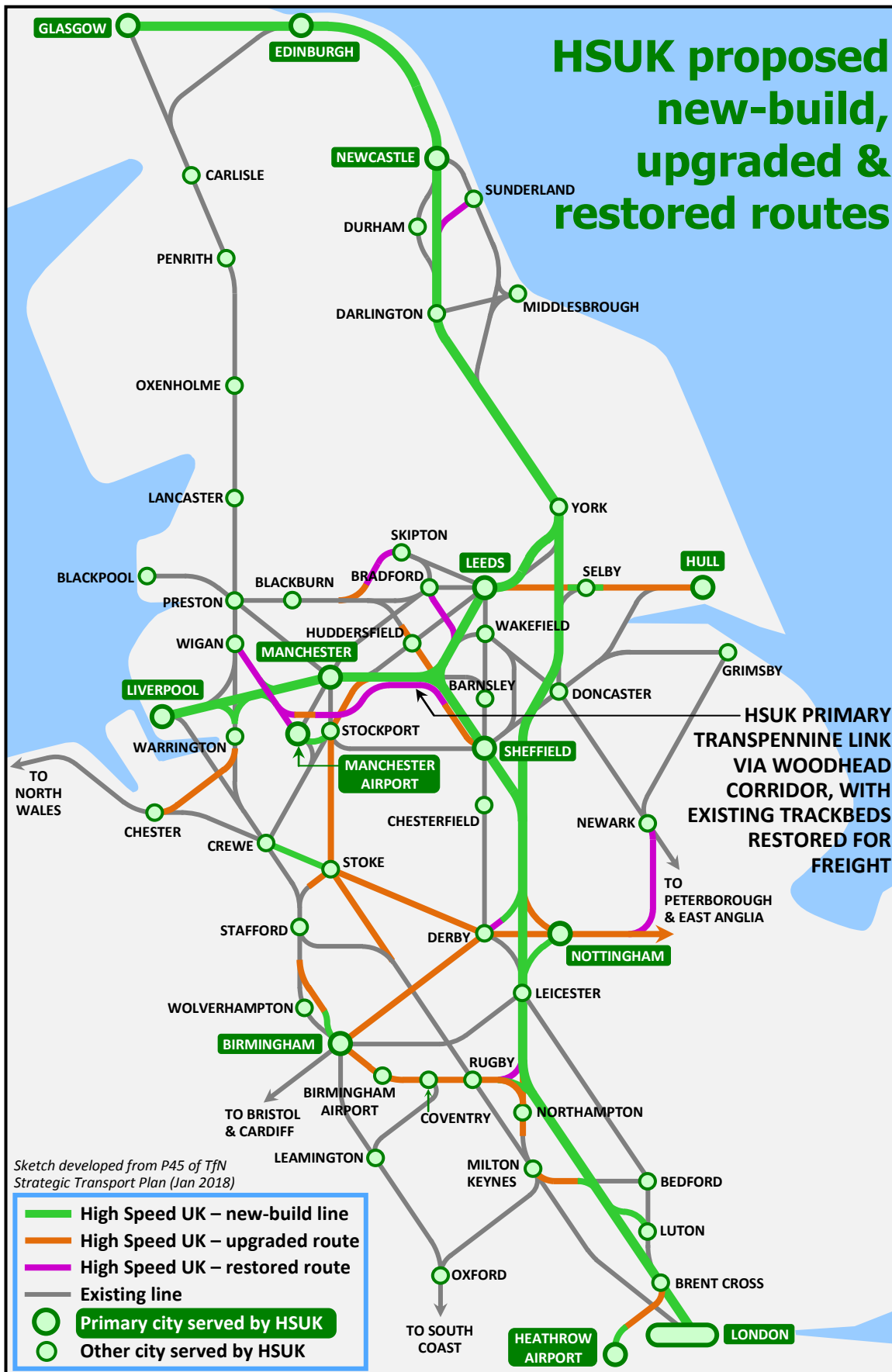
Figure B1 : HSUK 'Spine & Spur' network extending to all major UK conurbations
